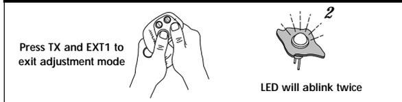
When the sensitivity adjustment procedure is completed, press and release the TX/Panic and the EXT-1/Valet buttons simultaneously. The status LED will blink twice and you will exit the adjustment mode. The system has now returned to the disarmed state.
