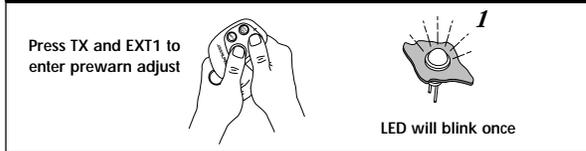
Within five seconds, press and immediately release (DO NOT HOLD) the TX/Panic and EXT-1/Valet buttons simultaneously. The status LED will illuminate once again. The system is now in the Impact Sensor Sensitivity Adjustment mode for the pre-warn field.
