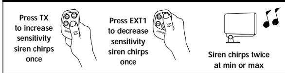
Press and release the TX/Panic button to increase the pre-warn sensitivity. Press and release the EXT-1/Valet button to decrease the pre-warn sensitivity. Each time the sensitivity is adjusted, the siren will chirp once. When the maximum or minimum sensitivity is reached, the siren will chirp twice. To test the pre-warn sensitivity level, strike the vehicle with a light impact. The status LED will blink once to indicate that the pre-warn sensitivity level has been exceeded.
